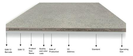
Details are printed on the edge of the tile as above. There is also information on the label over the plastic corner protector.
